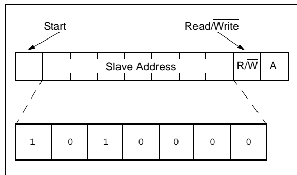
FIGURE 3-7: CONTROL BYTE ALLOCATION
