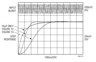
Figure 15. Step Responses with 60Hz Burst
