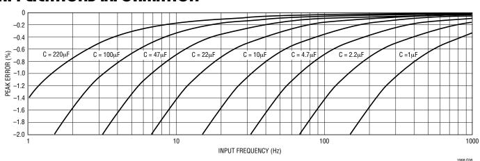
Figure 8. Peak Error vs Input Frequency with One Cap Averaging
