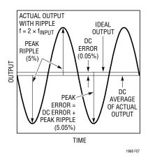
Figure 7. Output Ripple Exceeds DC Error
