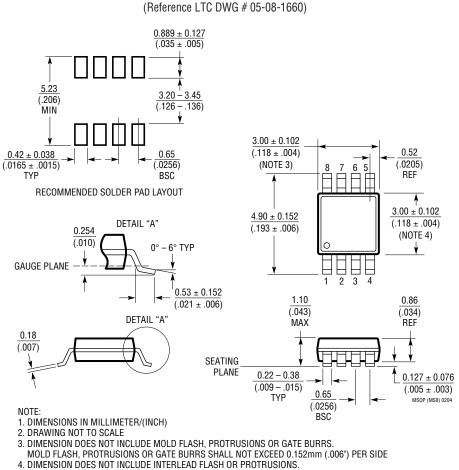
**MS8** Package 8-Lead Plastic MSOP
