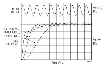
Figure 14. Step Responses with 10Hz Burst
