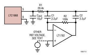
Figure 12. Buffered Post Filter
