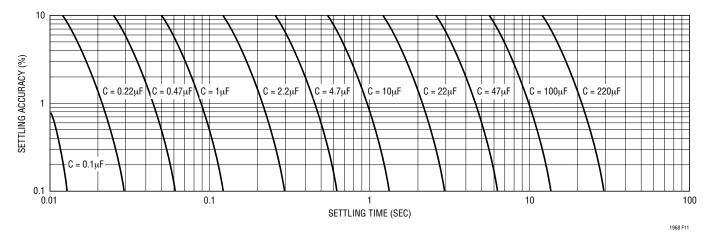
Figure 11. Settling Time vs Cap Value, One Cap Averaging
