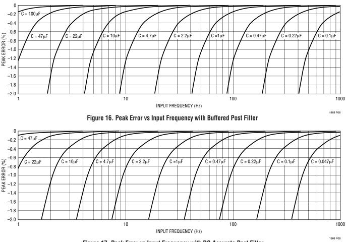
Figure 17. Peak Error vs Input Frequency with DC-Accurate Post Filter
