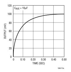
Figure 10a. LTC1968 Rising Edge with  $C_{AVE} = 10 \mu F$
