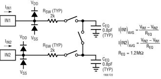
Figure 20. LTC1968 Equivalent Analog Input Circuit
