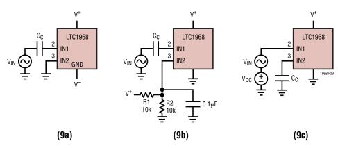
Figure 9. Single-Ended AC-Coupled Input Connection Alternatives
