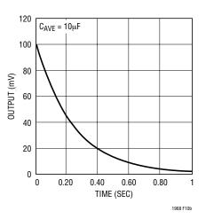
Figure 10b. LTC1968 Falling Edge with  $C_{AVE} = 10 \mu F$
