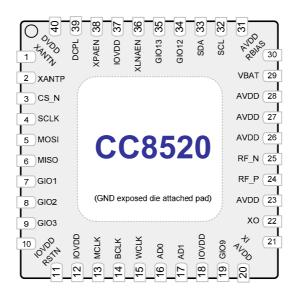
Figure 1 - CC8520 QFN Package Top View
