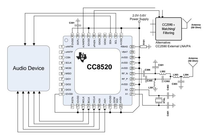
Figure 2 - CC8520 Application Circuit
