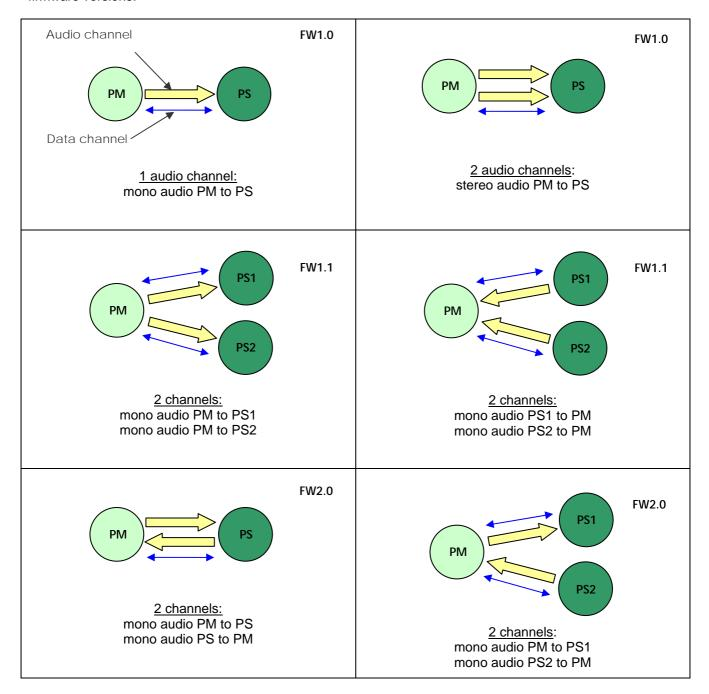
Figure 3 CC8520 topologies supported for different CC8520 FW revisions
