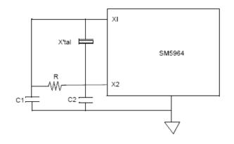
NOTE: Oscillation circuit may differs with different crystal or ceramic resonator in higher oscillation frequency which was due to each crystal or ceramic resonator has its own characteristics. User should check with the crystal or ceramic resonator manufacture for appropriate value of external components. Please see SM59264 application note for details.
