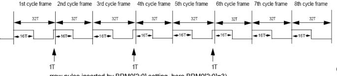
rrow pulse inserted by BRM0[2:0] setting, here BRM0[2:0]=3)
