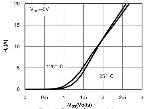
Figure 2: Transfer Characteristics
