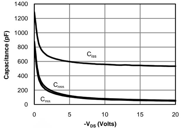
Figure 8: Capacitance Characteristics
