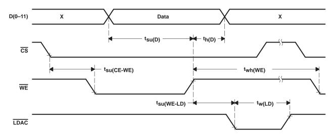
Figure 1. Timing Diagram
