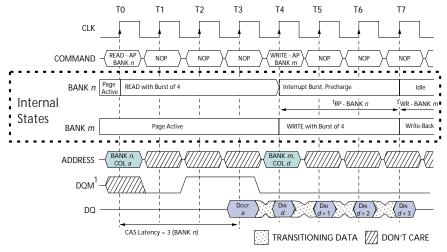
NOTE: 1. DQM is HIGH at T2 to prevent Dout-a+1 from contending with DIN-d at T4.
