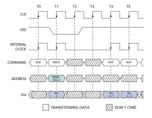
Clock suspend mode is exited by registering CKE HIGH; the internal clock and related operation will resume on the subsequent positive clock edge.
