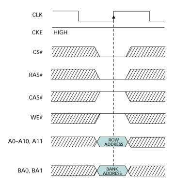
Figure 4 Example: Meeting  ${}^tRCD$  (MIN) When 2 <  ${}^tRCD$  (MIN)/ ${}^tCK \le 3$
