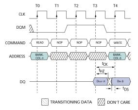
NOTE: A CAS latency of three is used for illustration. The READ command may be to any bank, and the WRITE command may be to any bank. If a burst of one is used, then DQM is not required.
