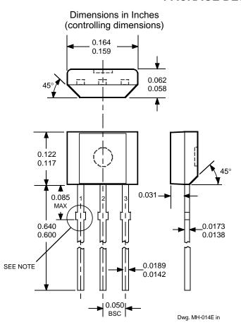
NOTES: 1. Tolerances on package height and width represent allowable mold offsets. Dimensions given are measured at the widest point (parting line).
