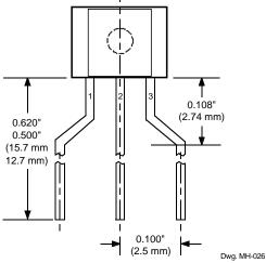
E: Lead-form dimensions are the nominals produced on the forming equipment. No dimensional tolerance is implied or guaranteed for bulk packaging (500 pieces per bag).
