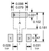
Pads 1, 2, 3, and A — Standard SOT89 Layout Pads 1, 2, 3, and B — Low-Stress Version
