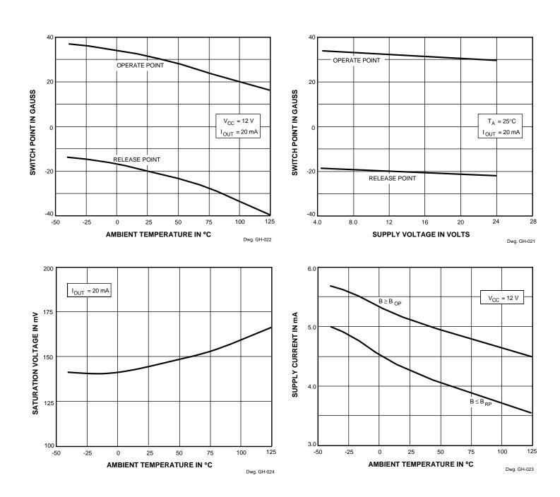
Powering up in the absence of a magnetic field (less than  $B_{OP}$  and higher than  $B_{RP}$ ) will allow an indeterminate output state. The correct state is warranted after the first excursion beyond  $B_{OP}$  or  $B_{RP}$ .
