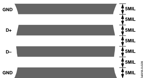
Figure 29. Arrangement of Signal Tracks
