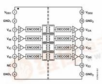
Figure 1. ADuM1400 Functional Block Diagram
