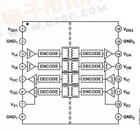
Figure 3. ADuM1402 Functional Block Diagram
