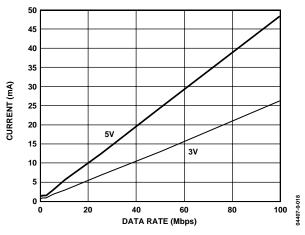
Figure 15. Typical ADuM1402 V<sub>DD1</sub> or V<sub>DD2</sub> Supply Current vs. Data Rate for 5 V and 3 V Operation
