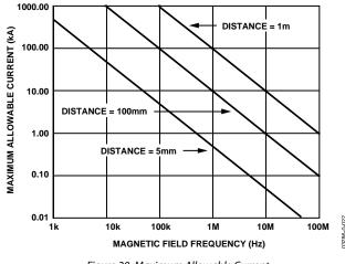
Figure 20. Maximum Allowable Current for Various Current-to-ADuM140x Spacings
