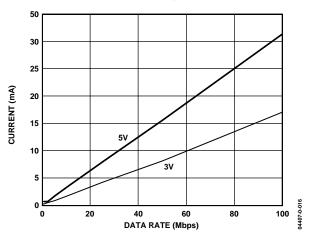
Figure 13. Typical ADuM1401 V<sub>DD1</sub> Supply Current vs. Data Rate for 5 V and 3 V Operation
