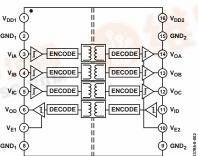
Figure 2. ADuM1401 Functional Block Diagram
