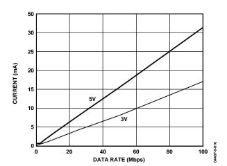
Figure 13. Typical ADuM2401 V<sub>DD1</sub> Supply Current vs. Data Rate for 5 V and 3 V Operation
