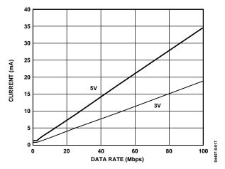
Figure 14. Typical ADuM2401 V<sub>DD2</sub> Supply Current vs. Data Rate for 5 V and 3 V Operation
