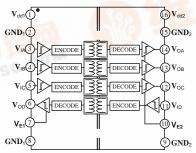
Figure 2. ADuM2401 Functional Block Diagram
