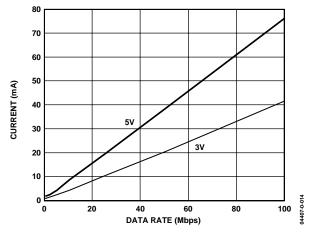
Figure 11. Typical ADuM2400  $V_{\rm DD1}$  Supply Current vs. Data Rate for 5 V and 3 V Operation
