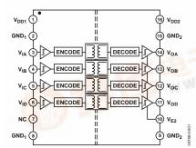
Figure 1. ADuM2400 Functional Block Diagram
