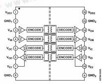
Figure 3. ADuM2402 Functional Block Diagram
