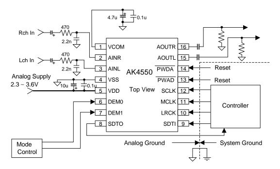
Figure 3. System Connection Diagram Example
