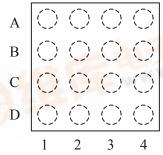
16-Ball STPBGA (4mm x 4mm) 14-Pin Flip Chip (100-mil x 100-mil) (*Not Shown*)
