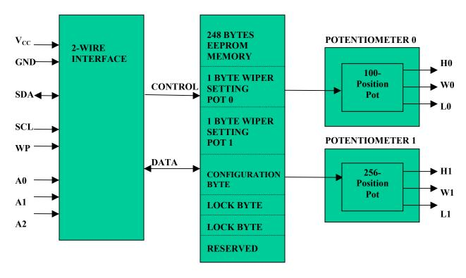
Up to eight DS1855s can be installed on a single 2-wire bus. Access to an individual device is achieved by using a device address that is determined by the logic levels of address pins A0 through A2. Additionally, the DS1855 will operate from 3V or 5V supplies. Three package options are available: 14-pin TSSOP, 16-ball STPBGA, and flip-chip package.
