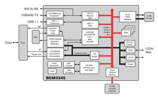
The BCM3345 combines an advanced QAM receiver; an advanced QAM transmitter; a complete DOCSIS/EuroDOCSIS Media Access Controller (MAC); a 140-MHz MIPS32 communication processor; a 16-bit, 100-MHz SDRAM interface; 10/100 Ethernet MAC with integrated transceiver and MII interface; and a USB 1.1 controller with integrated transceiver.
