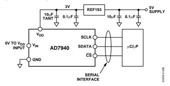
Figure 15. Typical Connection Diagram
