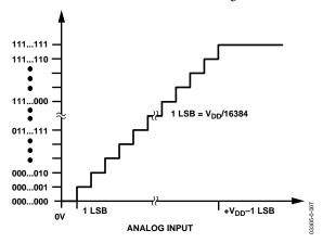
Figure 14. AD7940 Transfer Characteristic
