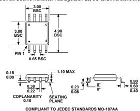
Figure 25. 8-Lead Micro Small Outline Package [MSOP] (RM-8). Dimensions shown in millimeters.
