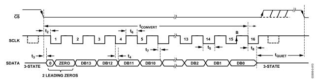
Figure 20. AD7940 Serial Interface Timing Diagram
