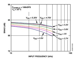
Figure 6. AD7940 SINAD vs. Analog Input Frequency for Various Supply Voltages at 100 kSPS
