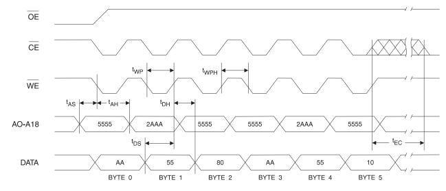
Note:  $\overline{OE}$  must be high only when  $\overline{WE}$  and  $\overline{CE}$  are both low.
