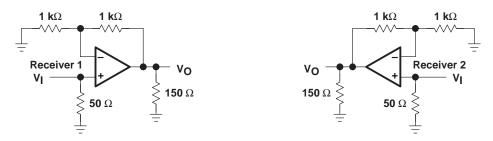
Figure 2. Receiver Input-to-Output Crosstalk Test Circuit
