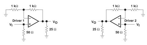
Figure 1. Driver Input-to-Output Crosstalk Test Circuit
