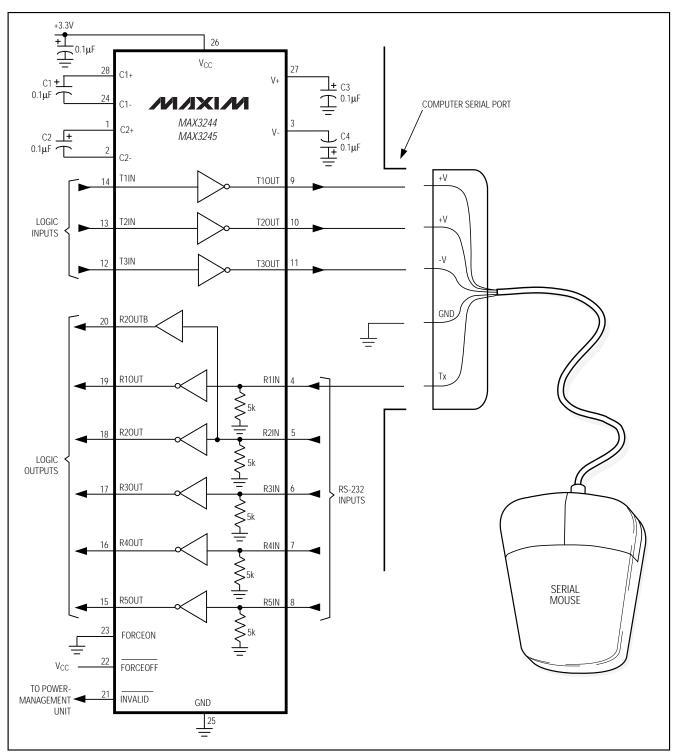
Figure 11b. Mouse Driver Test Circuit
