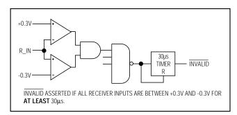
Figure 3a. INVALID Functional Diagram, INVALID Low
