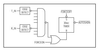
Figure 3c. AutoShutdown Plus Logic
