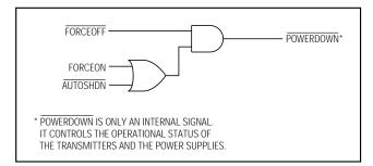
Figure 3d. Power-Down Logic
