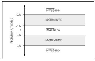
Figure 4a. Receiver Positive/Negative Thresholds for INVALID
