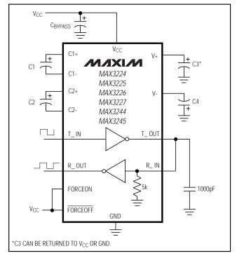
Figure 7. Loopback Test Circuit
