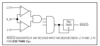
Figure 3b. INVALID Functional Diagram, INVALID High
