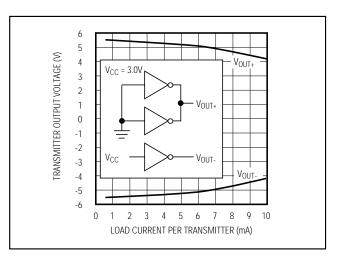
Figure 11a. MAX324\_ Transmitter Output Voltage vs. Load Current per Transmitter
