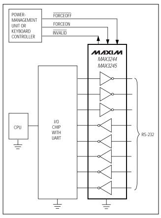
Figure 1. Interface Under Control of PMU
