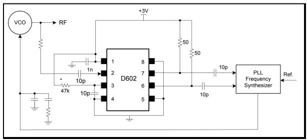
\* The 47kΩ resistor provides a DC offset that disables self oscillation in the absence of an RF input.
