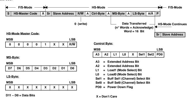
Figure 34. High-Speed Mode: Slave Receiver
