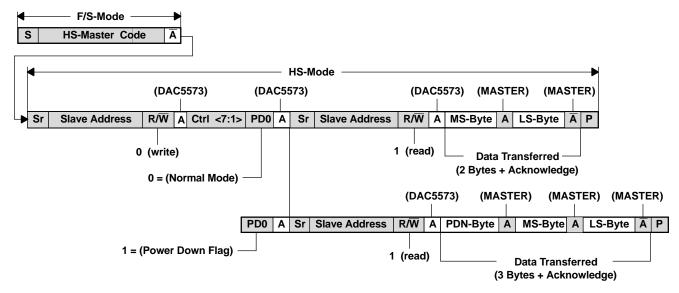
Figure 36. High-Speed Mode: Slave Transmitter
