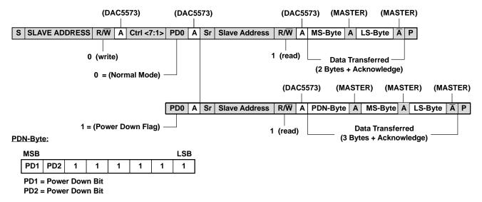
Figure 35. Standard and Fast Mode: Slave Transmitter
