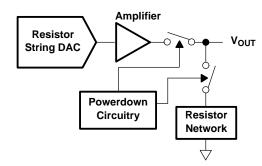
Figure 37. Output Stage During Power Down
