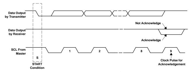
Figure 31. Acknowledge on the I<sup>2</sup>C Bus
