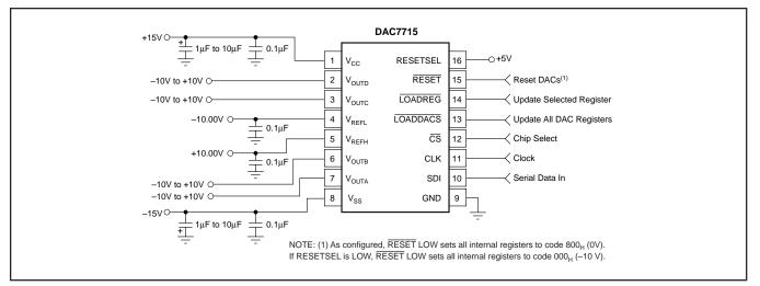
FIGURE 3 Basic Dual-Supply Operation of the DAC7715
