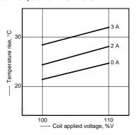
2-(2) Coil temperature rise 2 coil latching Tested sample: DS2Y-SL2-DC12V, 5 pcs. Measured portion: Inside the coil Ambient temperature: 21°C to 25°C 70°F to 77°F
