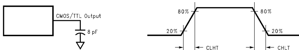
FIGURE 4. DS90CF384A/DS90CF364A (Receiver) CMOS/TTL Output Load and Transition Times
