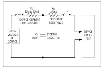
Figure 5a. IEC 1000-4-2 ESD Test Model
