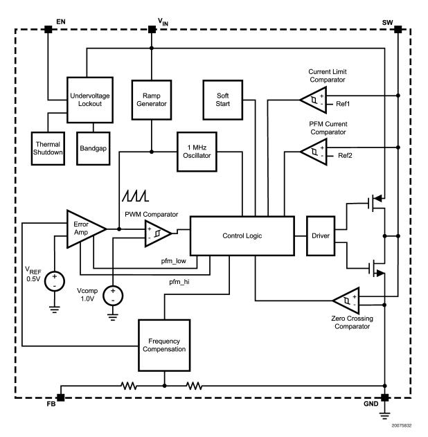
FIGURE 4. Simplified Functional Diagram
