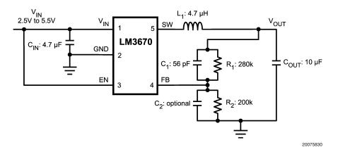
FIGURE 2. 1.2V - Adjustable Output Voltage - Typical Application Circuit
