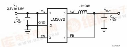
FIGURE 1. 1.8V - Fixed Output Voltage - Typical Application Circuit
