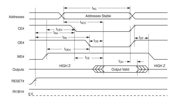
Figure II. Read Operation Timings
