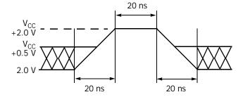
Figure 7. Maximum Negative Overshoot Waveform
