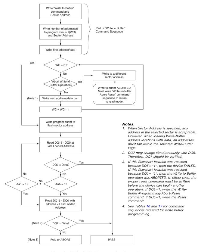
Figure I. Write Buffer Programming Operation
