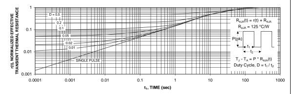
Figure 11. Transient Thermal Response Curve.
