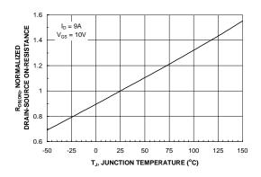
Figure 3. On-Resistance Variation with Temperature.
