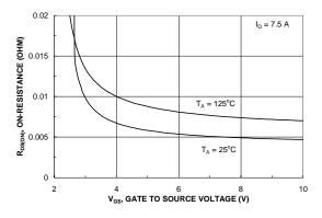
Figure 4. On-Resistance Variation with Gate-to-Source Voltage.
