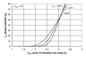
Figure 5. Transfer Characteristics.
