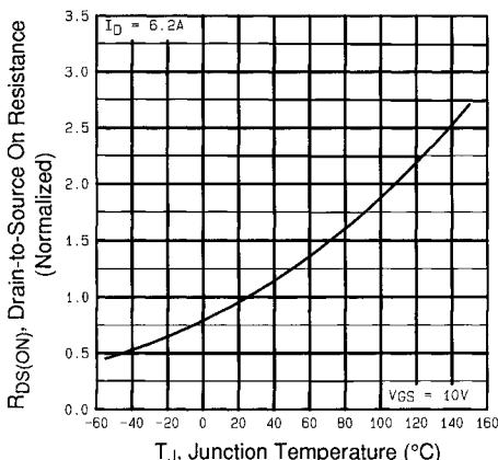
**Fig 4.** Normalized On-Resistance
