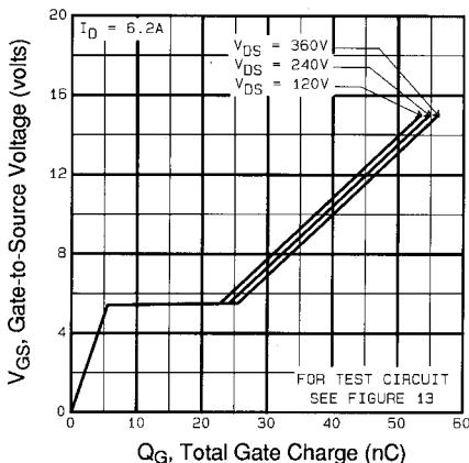
**Fig 6.** Typical Gate Charge Vs.
