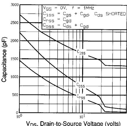
**Fig 5.** Typical Capacitance Vs.
