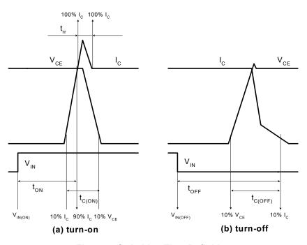
Figure 4. Switching Time Definition
