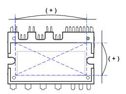
Figure 5. Flatness Measurement Position
