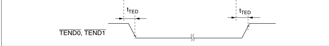
Figure 21-20 DMAC \overline{\text{TEND}} Output Timing
