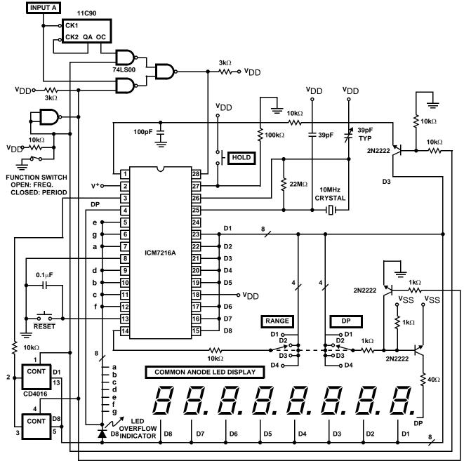
FIGURE 18. 100MHz FREQUENCY, 2MHz PERIOD COUNTER
