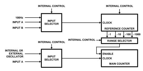
FIGURE 8. SIMPLIFIED BLOCK DIAGRAM OF FUNCTIONS IMPLEMENTATION
