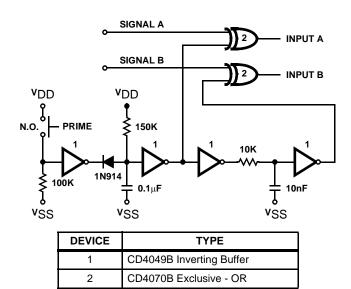
FIGURE 10. PRIMING CIRCUIT, SIGNALS A AND B BOTH HIGH OR LOW
