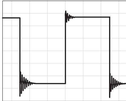
(b) C_L = 170 \text{ pF} , R_L = \text{NO LOAD}
