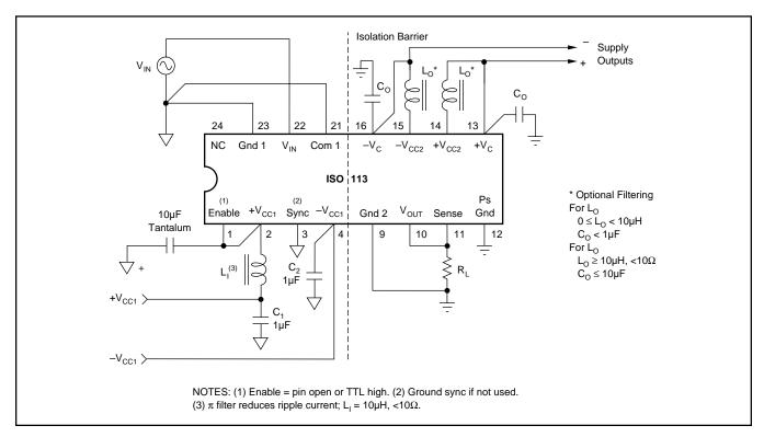
FIGURE 1. Signal and Power Connections.
