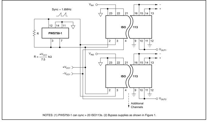
FIGURE 7. Synchronized-Multichannel Isolation.
