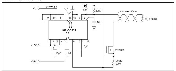
FIGURE 6. Isolated Current Loop Driver.
