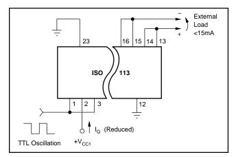
FIGURE 5. Reduced Power Dissipation.
