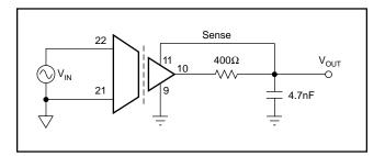
FIGURE 4. Ripple Reduction.
