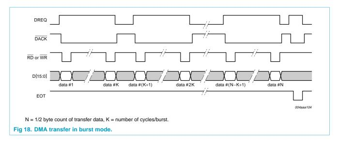
In Figure 17 and Figure 18, the hardware is configured such that DREQ is active HIGH and DACK is active LOW.
