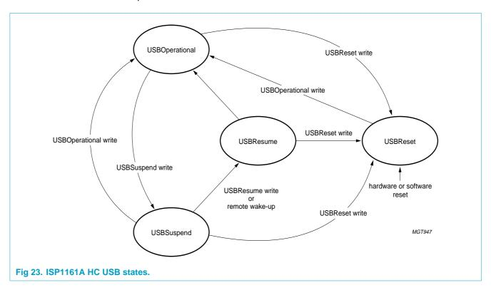
The USB states are reflected in the HostControllerFunctionalState field of the HcControl register (01H - read, 81H - write), which is located at bits 7 and 6 of the register.
