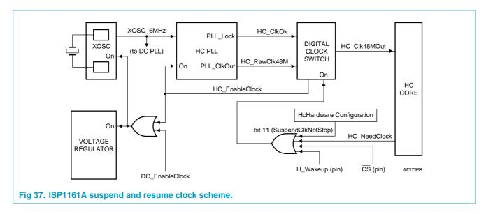
In suspended state, the device will consume considerably less power by turning off the internal 48 MHz clock, PLL and crystal, and setting the internal regulator to power-down mode. The ISP1161A suspend and resume clock scheme is shown in Figure 37.
