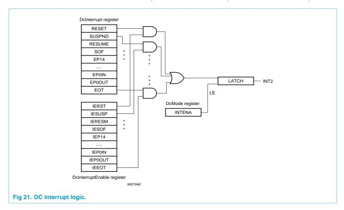
**Interrupt control:** Bit INTENA in the DcMode register is a global enable/disable bit. The behavior of this bit is given in Figure 22.
