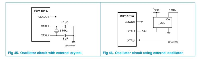
The 6 MHz oscillator frequency is multiplied to 48 MHz by an internal PLL. This frequency is used to generate a programmable clock output signal at pin CLKOUT, ranging from 3 MHz to 48 MHz.
