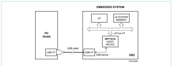
Fig 1. ISP1161A operating as a USB device.
