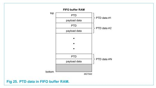
The PTD data structure is used by the HC to define a buffer of data that will be moved to or from an endpoint in the USB device. This data buffer is set up for the current frame (1 ms frame) by the HCD. The payload data for every transfer in the frame must have a PTD as a header to describe the characteristics of the transfer. PTD data is DWORD aligned.
