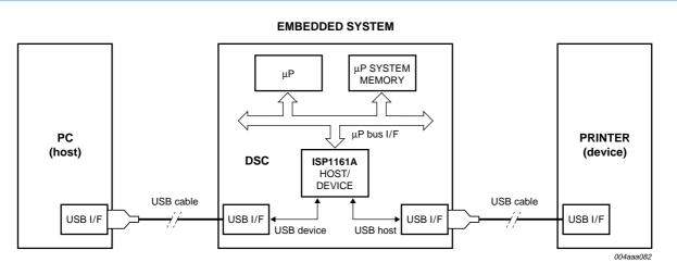
Fig 3. ISP1161A operating as both USB host and device simultaneously.
