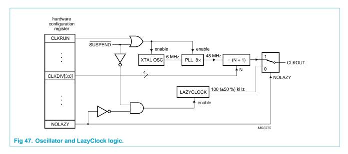
When ISP1161A's DC enters 'suspend' state (by setting and clearing bit GOSUSP in the DcMode register), outputs D\_SUSPEND and CLKOUT change state after approximately 2 ms delay. When NOLAZY = 0 the clock signal on output CLKOUT does not stop, but changes to the 100 kHz  $\pm$  50 % LazyClock frequency.
