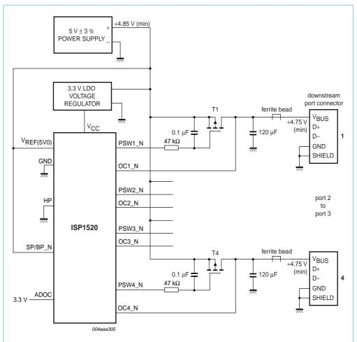
Fig 19. Self-powered hub; individual port power switching; individual overcurrent detection.
