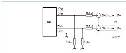
(1) Transmitter: connected to 50  $\Omega$  inputs of a high-speed differential oscilloscope. Receiver: connected to 50  $\Omega$  outputs of a high-speed differential data generator.
