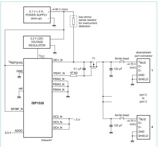
Fig 20. Self-powered hub; ganged port power switching; global overcurrent detection.
