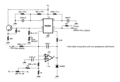
Figure 1. Precision Voltage-to-Frequency Converter, 100KHz Full-Scale
