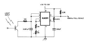
Figure 3. Light Intensity to Frequency Converter
