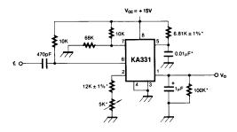
Figure 2. Simple Frequency-to-Voltage Converter, 10KHz Full-Scale
