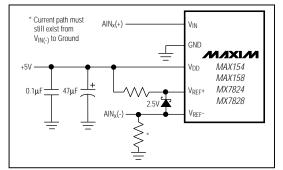
Figure 8d. Inputs Not Referenced to GND
