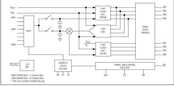
Figure 3. Functional Diagram
