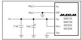
Figure 8c. Power Supply as Reference
