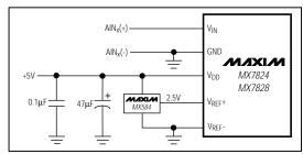
Figure 8b. External Reference +2.5V Full-Scale
