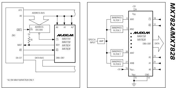
Figure 11. Simple Mode 0 Interface
