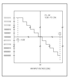
Figure 10b. Transfer Function for ±4V Input Operation
