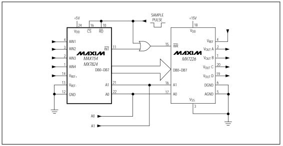
Figure 13. 4-Channel Fast Sample and Infinite Hold
