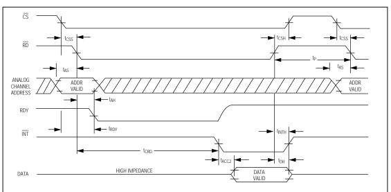
Figure 5. Mode 0 Timing Diagram
