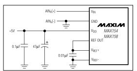
Figure 8a. Internal Reference (MAX154/MAX158 only)
