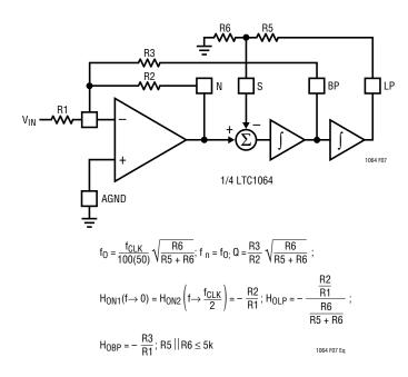
Figure 7. Mode 1b: 2nd Order Filter Providing Notch, Bandpass and Lowpass
