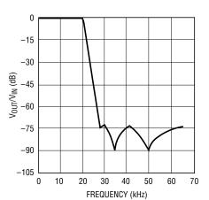
8TH ORDER CLOCK-SWEEPABLE LOWPASS ELLIPTIC ANTIALIASING FILTER MAINTAINS, FOR 0.1Hz  $\leq$   $f_{CUTOFF} \leq$  20kHz, A  $\pm$ 0.1dB MAX PASSBAND ERROR AND 72dB MIN STOPBAND ATTENUATION AT 1.5  $\times$   $f_{CUTOFF}$
