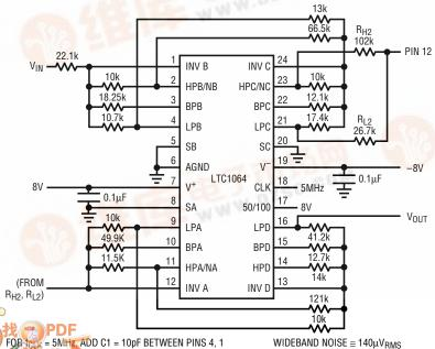
C2 = 10pF BETWEEN PINS 21, 24 C3 = 27pF BETWEEN PINS 9, 12
