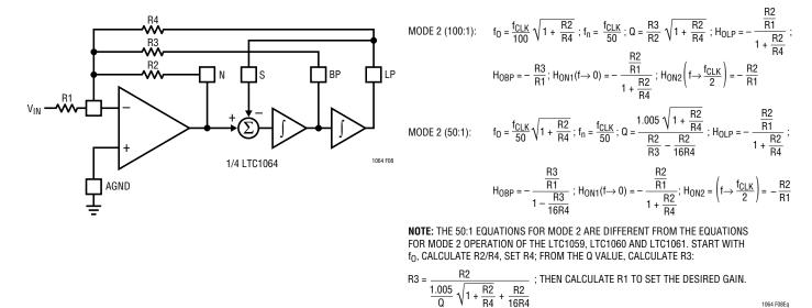
Figure 8. Mode 2: 2nd Order Filter Providing Notch, Bandpass and Lowpass
