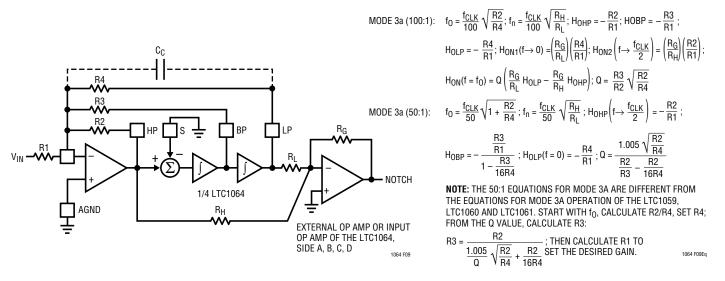
Figure 9. Mode 3a: 2nd Order Filter Providing Highpass, Bandpass, Lowpass and Notch
