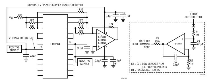
Figure 3. Buffering the Output of a 4th Order Bandpass Realization
