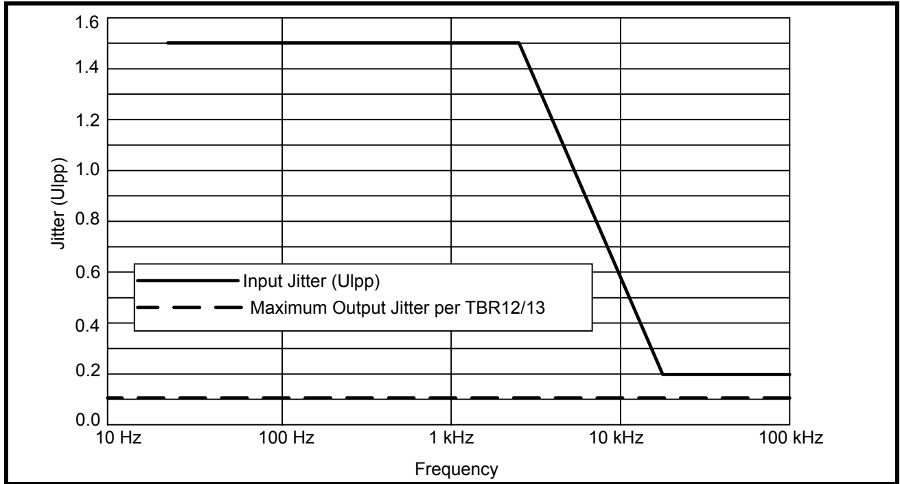
Figure 21: LXT318 Jitter Attenuation Performance (Typical—Measured Against TBR12/13)
