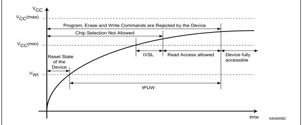
Table 6. Power-Up Timing and  $V_{WI}$  Threshold
