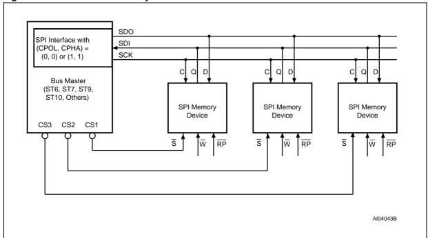
Note: The Write Protect  $(\overline{W})$  signal should be driven, High or Low as appropriate.
