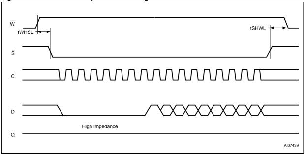
Figure 24. Output Timing
