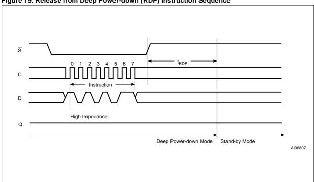
Figure 19. Release from Deep Power-down (RDP) Instruction Sequence
