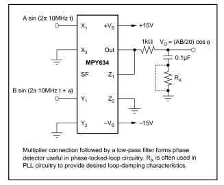
FIGURE 6. Phase Detector.
