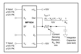
FIGURE 3. Conversion of Output to Current.
