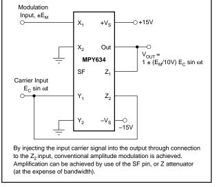
FIGURE 9. Linear AM Modulator.
