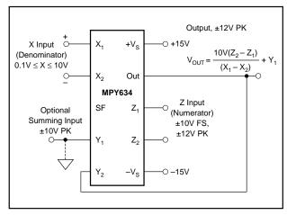
FIGURE 4. Basic Divider Connection.
