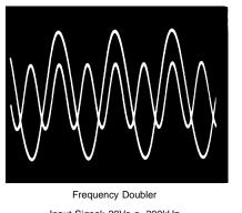
Input Signal: 20Vp-p, 200kHz Output Signal: 10Vp-p, 400kHz
