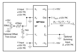
FIGURE 2. Basic Multiplier Connection.
