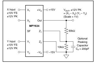
FIGURE 1. Connections for Scale-Factor of Unity.
