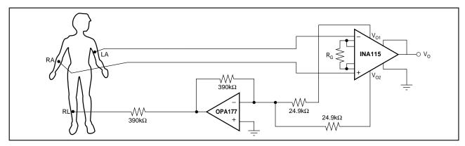
FIGURE 7. ECG Amplifier with Right Leg Drive.
