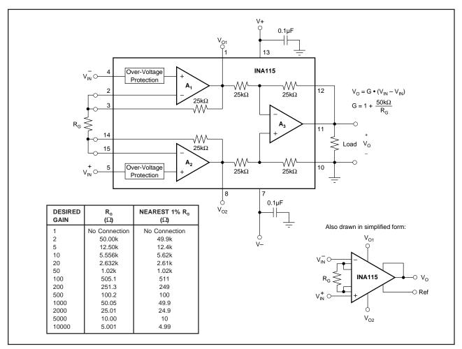
FIGURE 1. Basic Connections.
