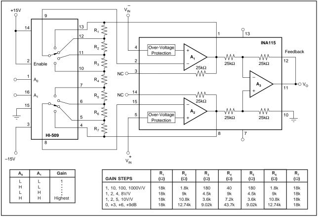
FIGURE 3. Switched-Gain Instrumentation Amplifier (improved gain drift).
