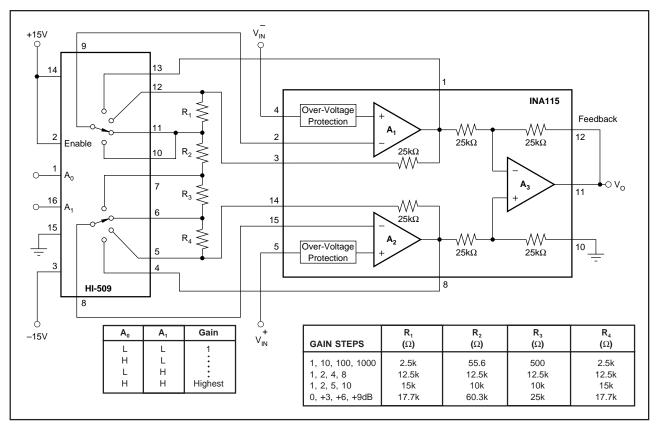
FIGURE 2. Switched-Gain Instrumentation Amplifier (minimum components).
