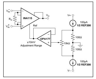
FIGURE 4. Optional Trimming of Output Offset Voltage.
