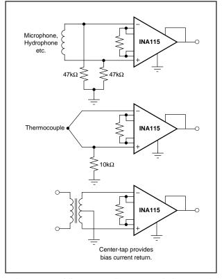
FIGURE 5. Providing an Input Common-Mode Current Path.
