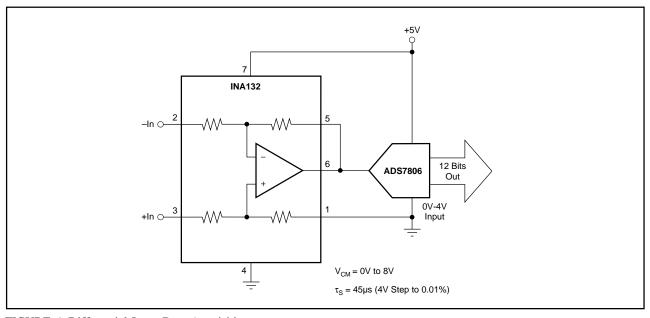
FIGURE 6. Differential Input Data Acquisition.
