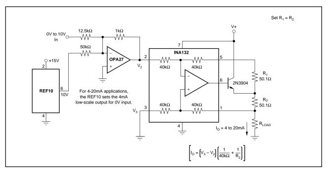
FIGURE 7. Precision Voltage-to-Current Conversion.
