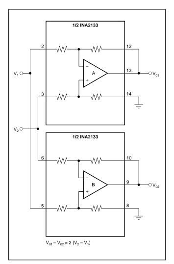
FIGURE 18. Differential Output Difference Amplifier.
