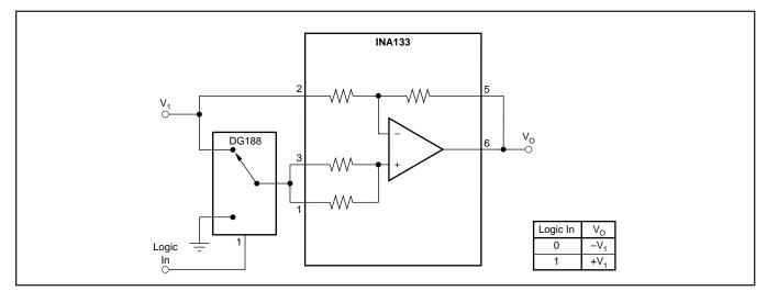
FIGURE 21. Digitally Controlled Gain of ±1 Amplifier.
