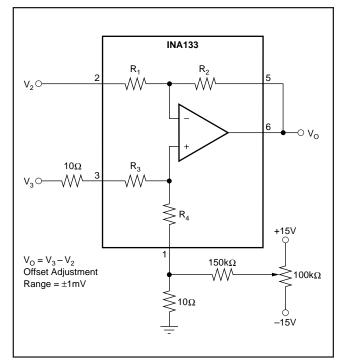
FIGURE 2. Offset Adjustment.
