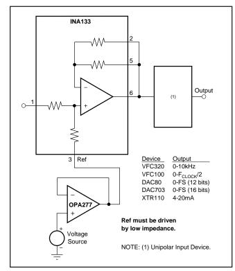
FIGURE 11. Precision Bipolar Offsetting.
