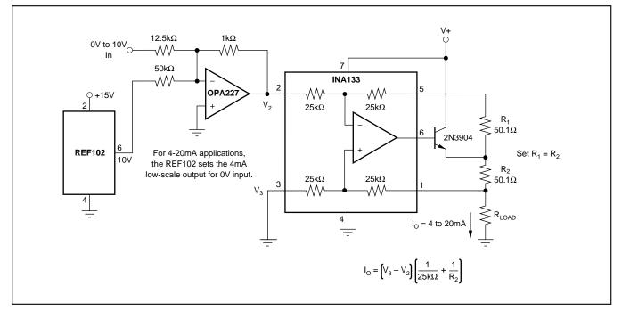
FIGURE 25. Precision Voltage-to-Current Conversion.
