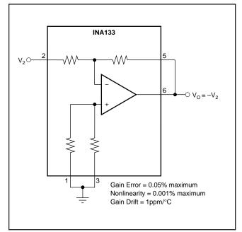
FIGURE 6. Precision Unity-Gain Inverting Amplifier.
