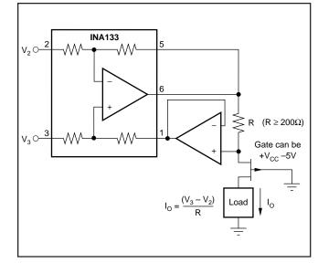
FIGURE 19. Isolating Current Source with Buffering Amplifier for Greater Accuracy.
