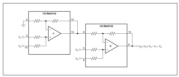
FIGURE 14. Precision Summing Instrumentation Amplifier.
