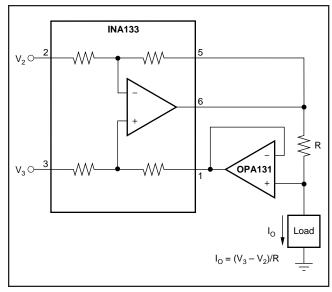
FIGURE 16. Differential Input Voltage-to-Current Converter for Low  $I_{OUT}$ .
