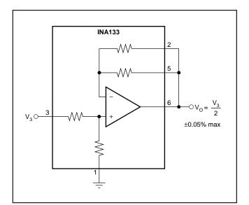
FIGURE 8. Precision Gain = 1/2 Amplifier.
