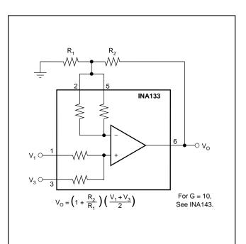
FIGURE 12. Precision Summing Amplifier with Gain.
