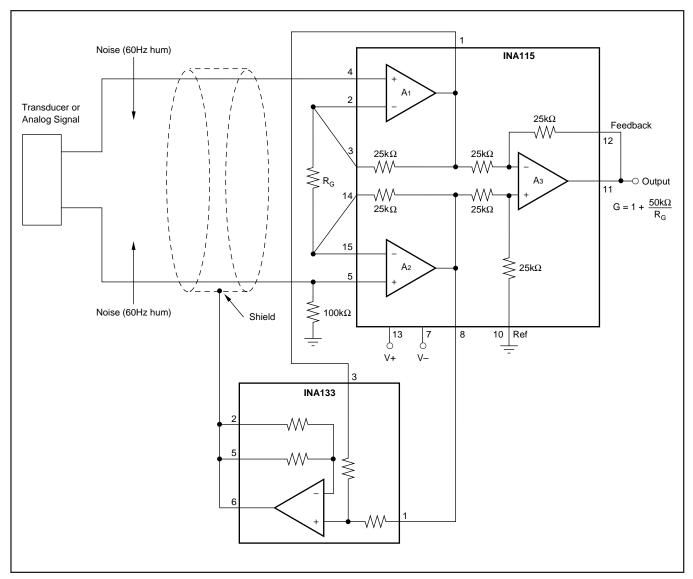
FIGURE 13. Instrumentation Amplifier Guard Drive Generator.
