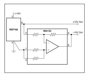
FIGURE 23. ±10V Precision Voltage Reference.
