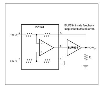
FIGURE 24. High Output Current Precision Difference Amplifier.
