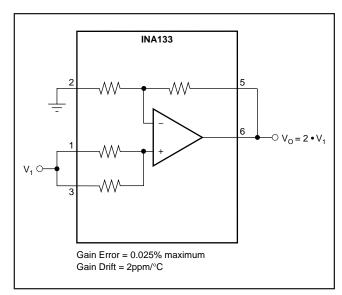
FIGURE 7. Precision Gain = 2 Amplifier.
