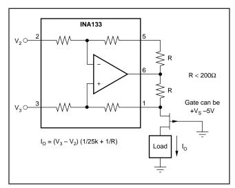
FIGURE 17. Isolating Current Source.
