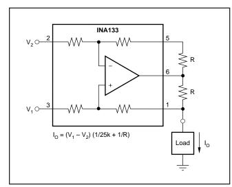
FIGURE 15. Precision Voltage-to-Current Converter with Differential Inputs.
