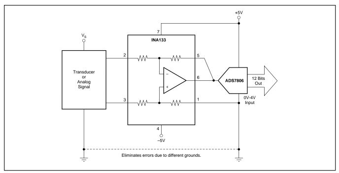
FIGURE 20. Differential Input Data Acquisition.
