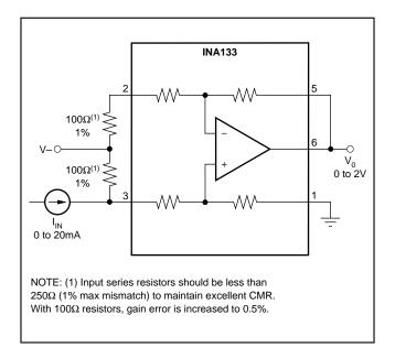
FIGURE 4. Current Receiver with Compliance to Rails.
