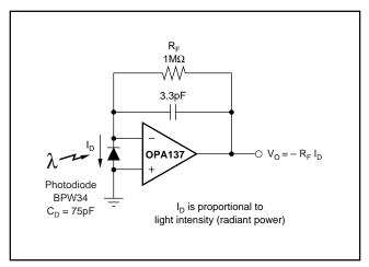
FIGURE 3. Photodetector Amplifier.
