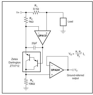
FIGURE 2. High-Side Current Monitor.
