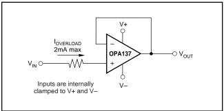
FIGURE 1. Input Current Protection for Voltages Exceed-
