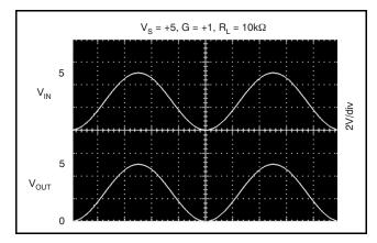
Figure 23. Rail-to-Rail Input and Output
