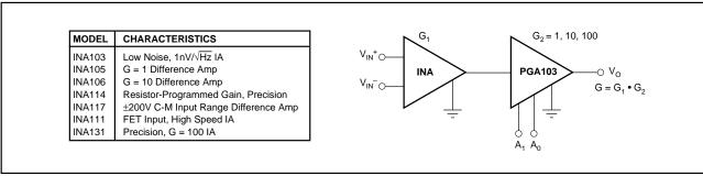
FIGURE 6. Instrumentation Amplifier with Programmable Gain Output Amp.
