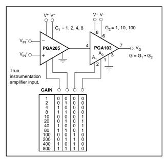
FIGURE 5. Wide Input Voltage Range Amplifer.
