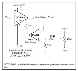
FIGURE 3. Offset Voltage Trim Circuit.
