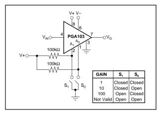
FIGURE 2. Switch or Jumper-Selected Gains.
