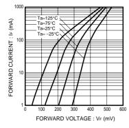
Fig.1 Forward Temperature Characteristics
