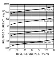
Fig.2 Reverse Temperature Characteristics
