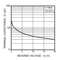
Fig.3 Capacitance Between Terminals Characteristics
