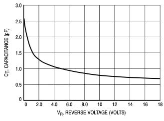
Figure 4. Typical Capacitance
