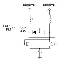
To tune the VCO the designer only needs to calculate the value of the inductors connected to pins 18 and 20 (RESNTR- and RESNTR+). The inductor value is determined by the following equation.
