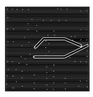
Evaluation Board Layout 915MHz Board Size 2.0" x 2.0"
